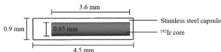
**Figure 2.** The microSelectron HDR  $^{192}\text{Ir}$  source as modeled using the Geant4 package.
