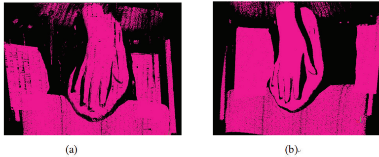
Fig. 6. The effect of 3D reconstruction. (a) The effect of 3D reconstruction without global phase filter. (b) The effect of 3D reconstruction after global phase filter.
