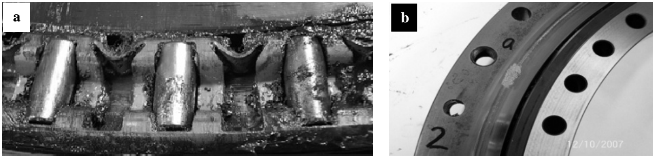
Fig. 14. Slew bearing damage: (a) a view of damaged rollers in the axial row; (b) outer raceway damage.
