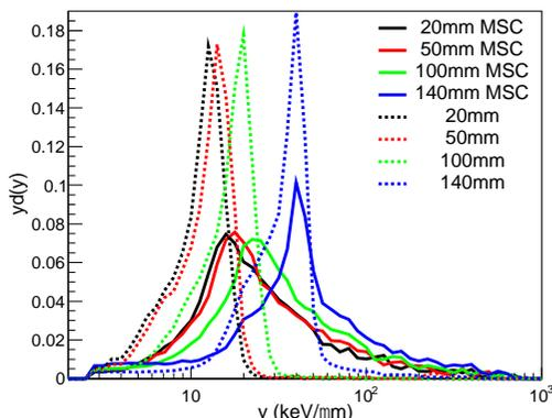
Figure 4. Comparison of microdosimetric spectra measured with the Bridge in a  $^{12}\text{C}$  ion broad beam (dashed lines) and MBRT field (solid lines) at varying depths in a water phantom.
