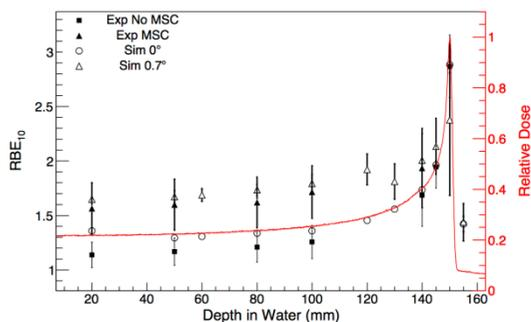
Figure 5.  $\text{RBE}_{10}$  values calculated from microdosimetric spectra measured with the Bridge microdosimeter detector from experiment and Geant4 simulation.
