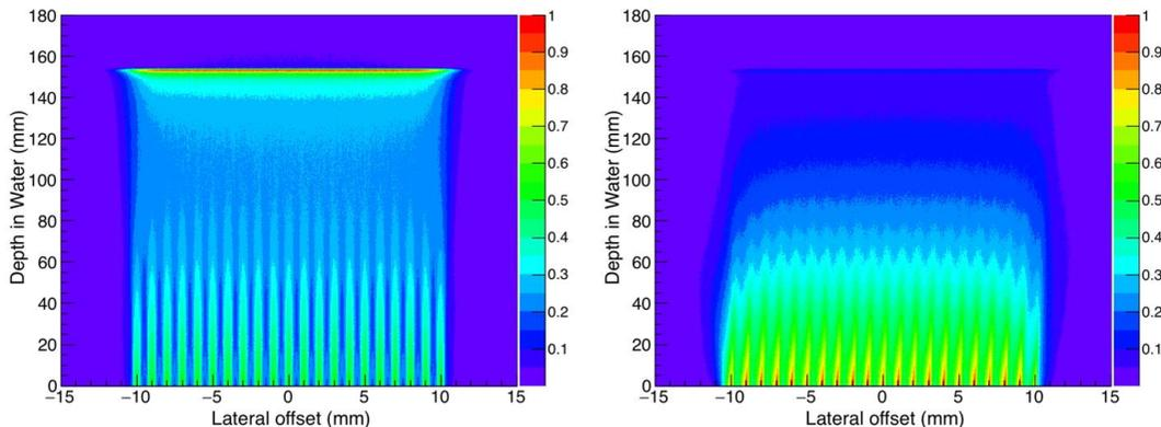
Figure 8. Simulated relative physical dose scored in a water phantom for perfect MSC alignment (left) and for a  $0.7^\circ$  misalignment (right) relative to the central beam axis.
