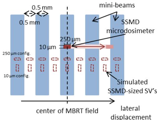
Figure 3. MSC and SSMD setup, the SSMD detector is represented by the solid box that was positioned at various lateral positions in the field. The dashed boxes represent the simulated SSMD-sized water volumes with two scoring orientations.
