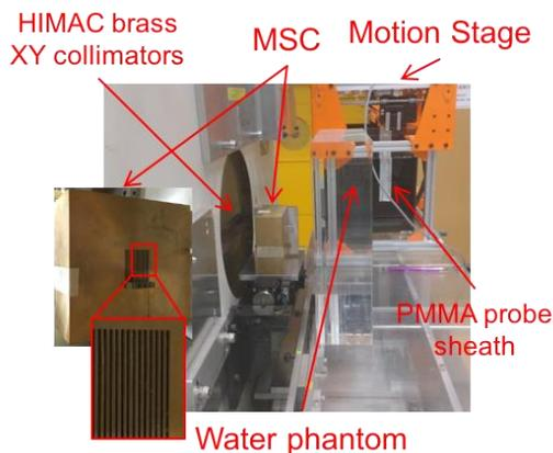
Figure 2. MSC and experimental setup
