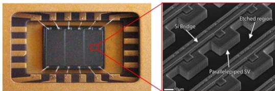
Figure 1. Bridge microdosimeter and scanning electron microscope image of sensitive volumes (right)
