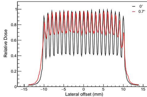
Figure 7. Simulated lateral dose profile of MBRT field at a depth of 20 mm in water for  $0^\circ$  and  $0.7^\circ$  MSC alignment relative to the beam axis.
