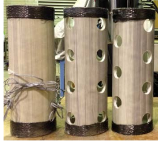
Fig. 2 – GFRP Tubes (solid tube, axially perforated tube, and diagonally perforated tube)
