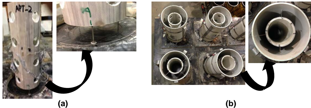
Fig. 3 – Layout of GFRP tubes: (a) 20 mm cover at bottom and (b) 30 mm cover on the sides
