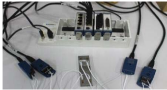
Figure 9. Strain gauge measurement devices
