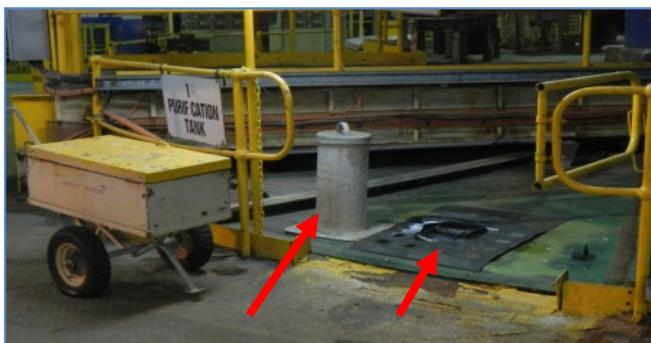
Image 2: As<sub>2</sub>O<sub>3</sub> trolley, chute and sample opening (Roseberg 2014)
