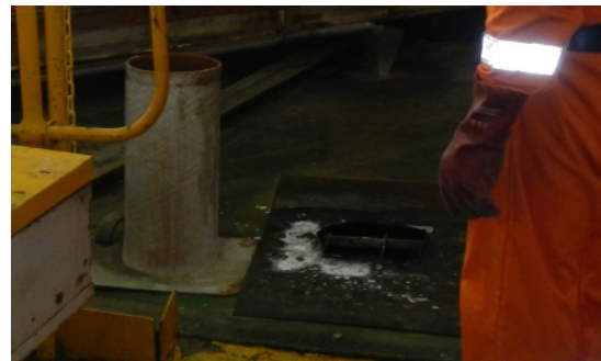
Image 5: Grate used to add arsenic (Roseberg, 2014)
