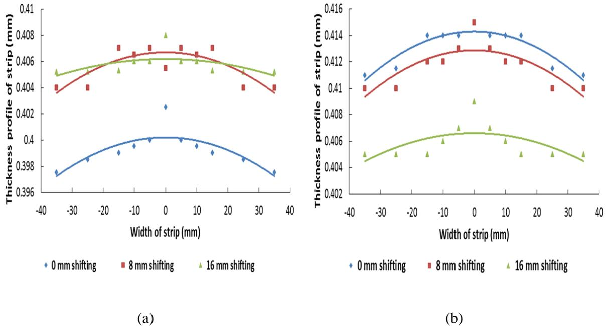
Fig. 4 Strip profile for different crossing angle and shifting values in a symmetrical rolling. (a) 0.5° crossing angle and (b) 1.0° crossing angle
