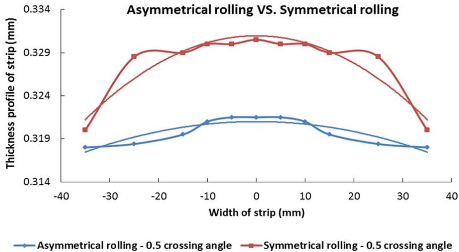
Fig. 2 Strip profile in asymmetrical and symmetrical rolling
