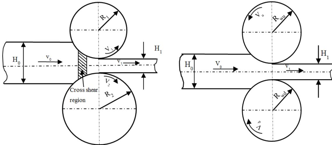
Fig. 1 Strip rolling process (a) asymmetrical rolling, (b) symmetrical rolling
