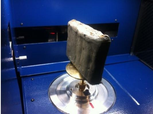
Figure 3 Soil-drain sample after confinement being scanned in the micro-CT chamber
