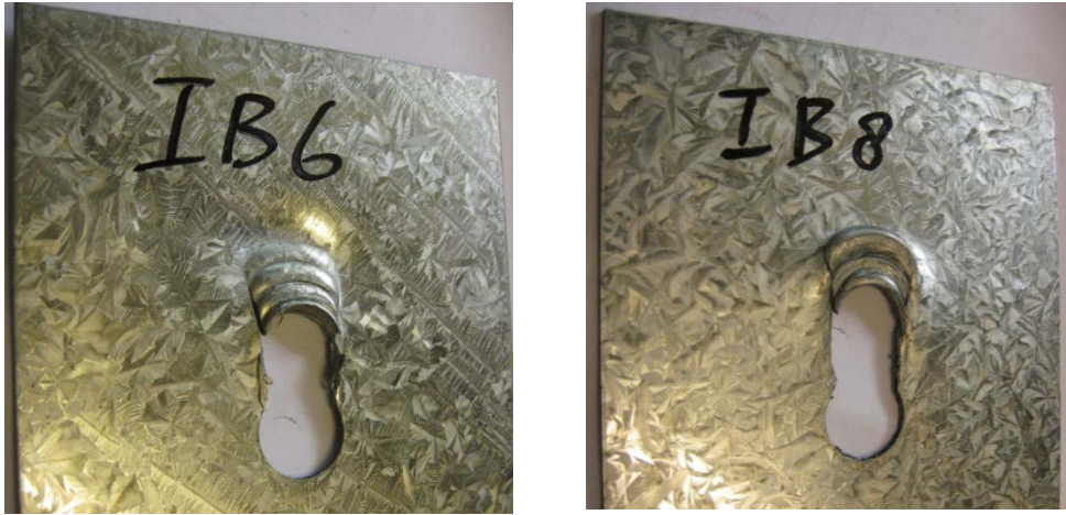
Figure 3 Failed specimens IB6 and IB8
