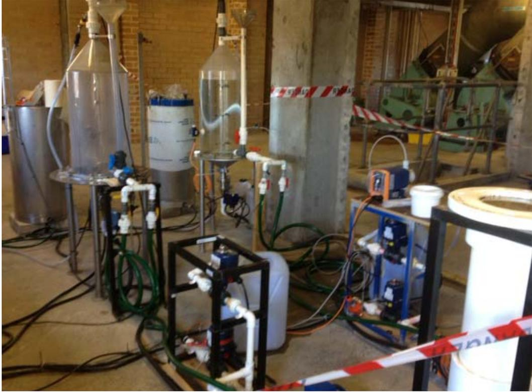
**Figure S1:** The pilot anaerobic digester.
