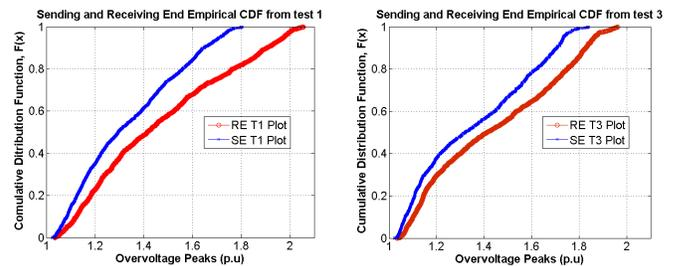
Fig. 3. CDF for Test 1 and Test 3 energisation schemes
