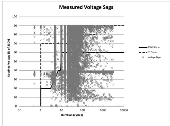
Figure 11: Measured Voltage Sags Plotted on Depth-Duration Plane
