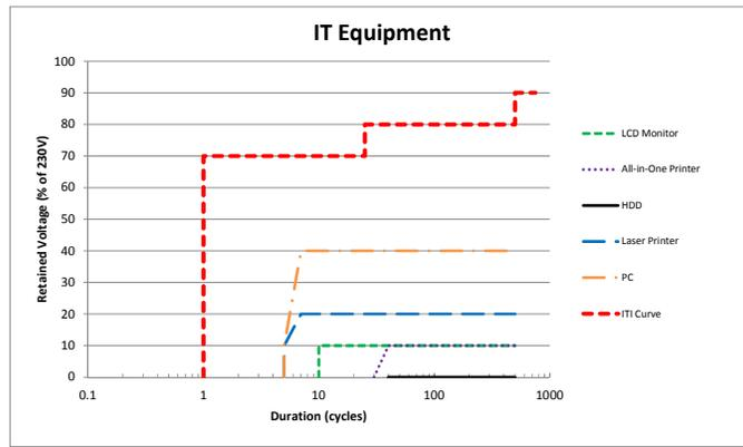
Figure 2: Voltage Sag Susceptibility Envelopes for IT Equipment
