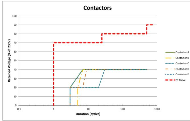
Figure 6: Voltage Sag Susceptibility Envelopes for Contactors
