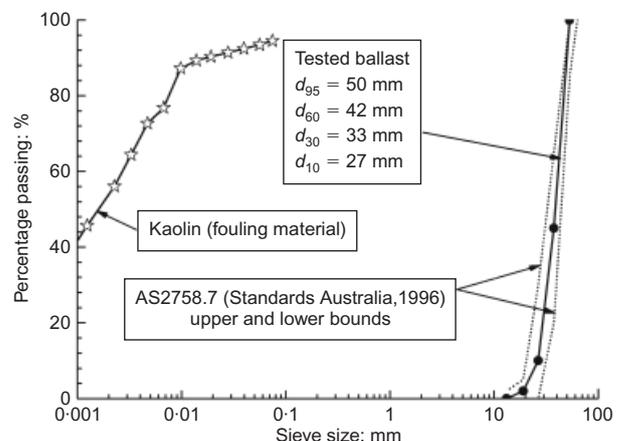
Fig. 1. Particle size distribution of test materials
