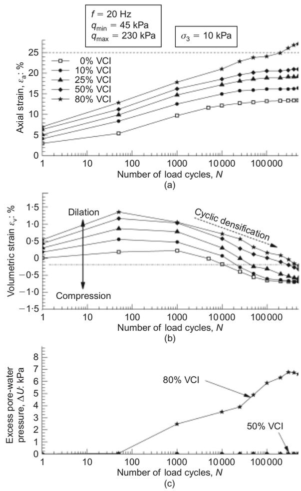
Fig. 3. Strain response under cyclic loading: (a) axial strain,  $\epsilon_a$ ; (b) volumetric strain,  $\epsilon_v$ ; (c) excess pore-water pressure measured at the middle of the specimen, as a function of the number of load cycles,  $N$
