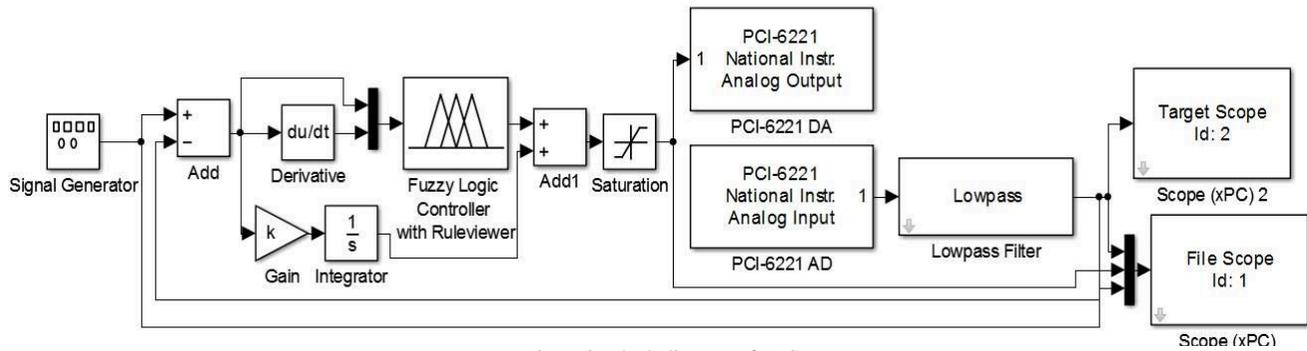
Figure 3. Block diagram of FLC
