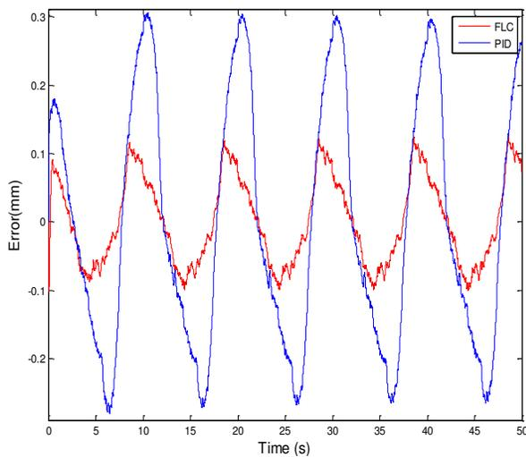
Figure 6. Tracking error of FLC and PID controller
