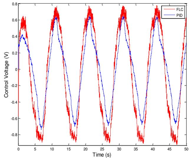
Figure 7. Control voltage of FLC and PID controller
