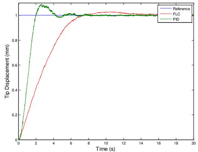
Figure 8. Comparison of the step responses with FLC and PID controller
