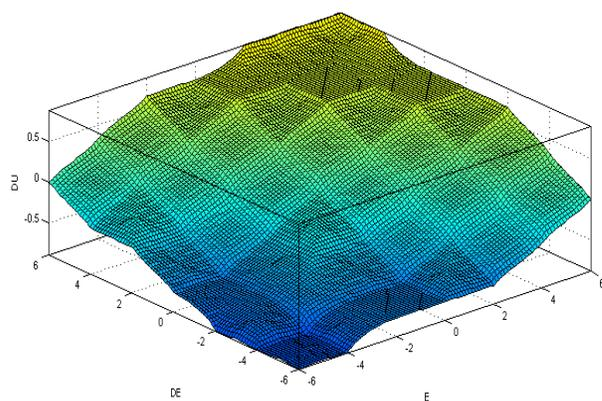
Figure 2. Fuzzy controller output surface
