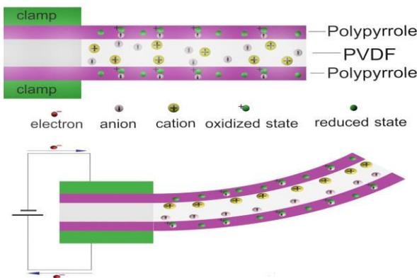
Figure 1. Actuation mechanism of the trilayer conjugated polymer actuator
