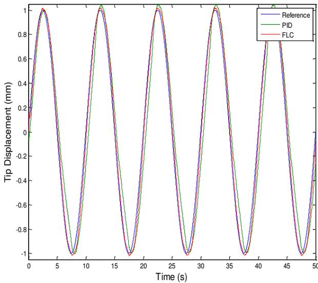
Figure 5. Comparison of displacement of CPA for sinusoidal signal
