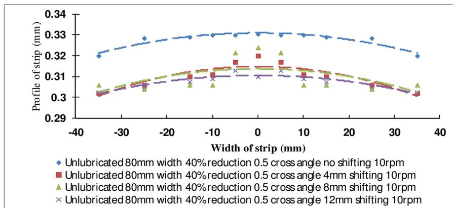
Figure 5. Thickness distribution at various work rolls crossing and shifting values
