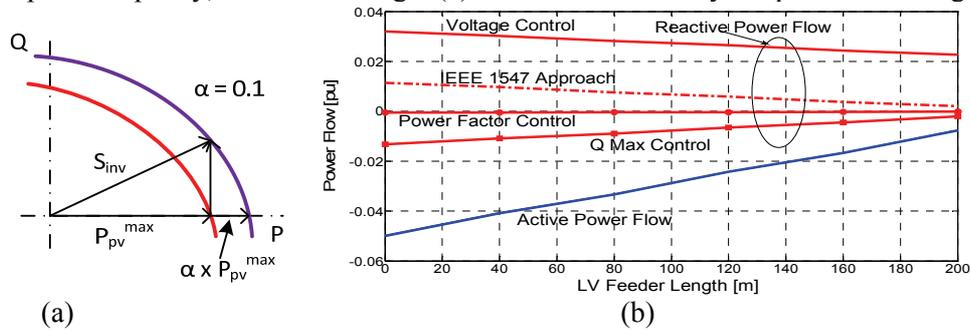
Fig. 6: Application of control strategies: (a) PV inverter capability (b) Reactive power flow in LV feeder
