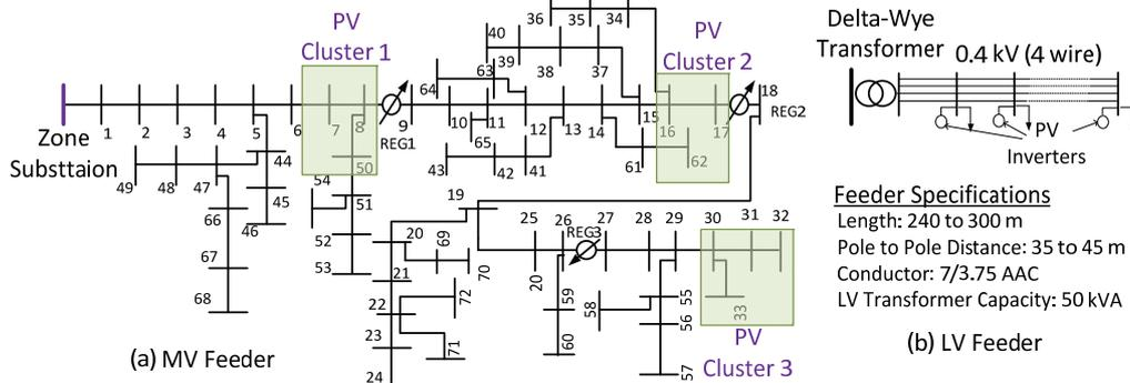
Fig. 5: Test feeder (a) 11 kV network (b) 0.4 kV LV feeder
