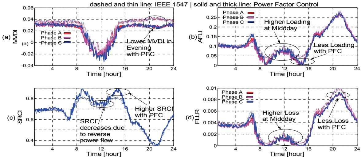
Fig. 8: Daylong variations of network performance indices with changing feeder loads and PV generations
