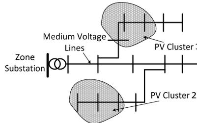
Fig. 3: Location of PV clusters in distribution feeders
