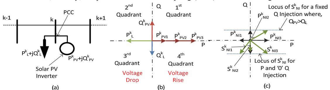
Fig. 1: Variation of net PQ injection (a) simple system diagram of an arbitrary phase of three phase LV feeder (b) four-quadrant PQ model for  $k^{\text{th}}$  system node (c) net P-Q injection for  $k^{\text{th}}$  system node
