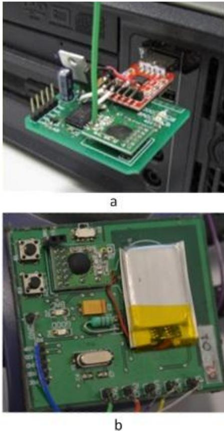
Figure 10. a. TENS transmitter. b. USB receiver
