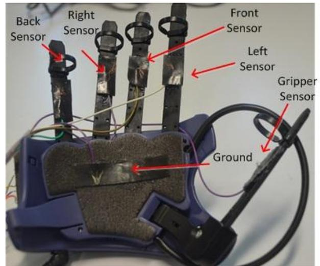
Figure 9. TENS electrodes fitted to data glove.
