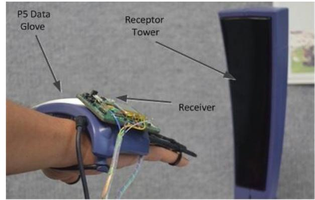
Figure 8. Data Glove with feedback unit and receptor tower.
