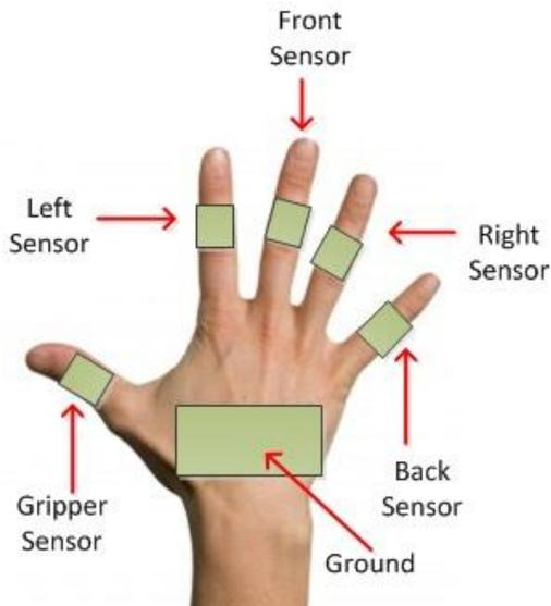
Figure 11. Position of the feedback electrodes
