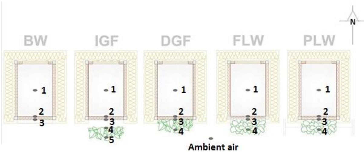
Figure 5: Plan layout (top view) - Location of 21 thermocouples across the five test cells
