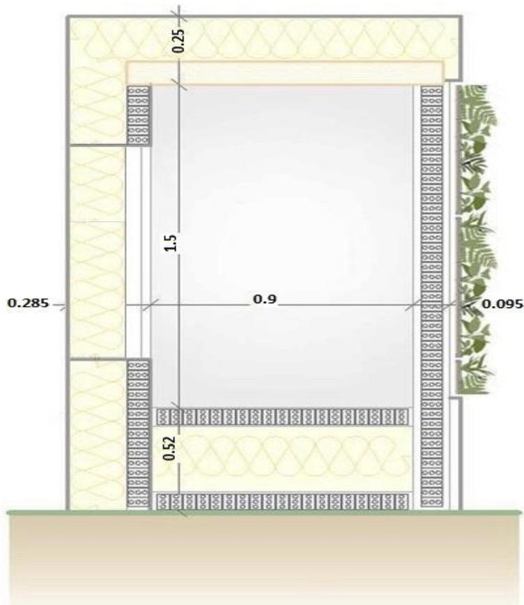
Figure 2: Cross section of the test cell structure
