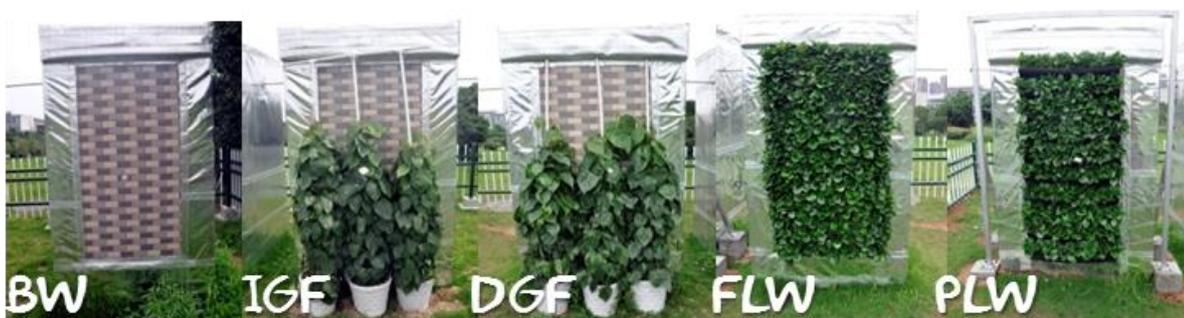
Figure 1: An overview of the five test cells and abbreviations used for the wall types
