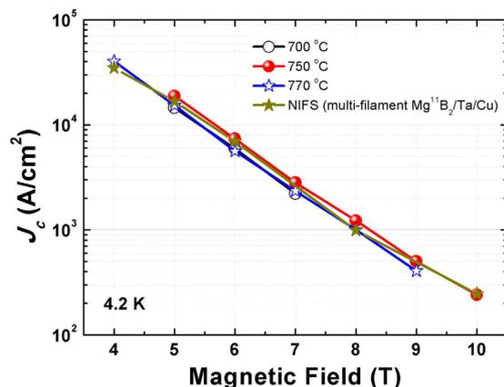
**Figure 1.** Transport  $J_c$  -  $B$  performance at 4.2 K of  $\text{Mg}^{11}\text{B}_2$  wires using amorphous  $^{11}\text{B}$  isotope as the boron source. Results from NIFS are also plotted for reference. No transport  $I_c$  was detected in the wire treated at 800 °C.
