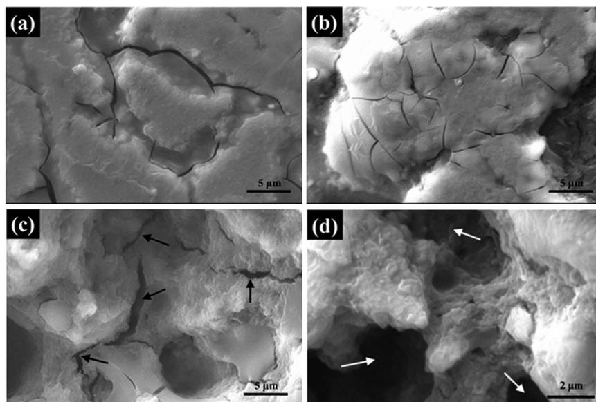
**Figure 4.** SEM micrographs of cross-sections of  $\text{Mg}^{11}\text{B}_2$  wires sintered at (a) 700 °C, (b) 750 °C, and (c) 800 °C. Evolution of the surface morphology is clearly shown. Black arrows indicate big cracks. (d) SEM image of the wire sintered at 800 °C under higher magnification. White arrows indicate porous structure in the sample sintered at 800 °C.
