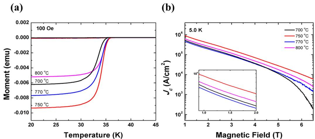
**Figure 3.** (a) Temperature dependence of the ZFC and FC dc magnetization measured in a field of 100 Oe. (b) Field dependence of the magnetic  $J_c$  at 5.0 K on the logarithmic scale (with the inset showing an enlargement of the  $J_c(H)$  at low fields) for all samples.
