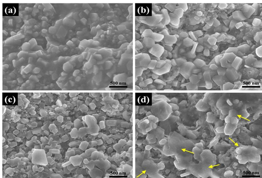
**Figure 5.** High-resolution SEM micrographs of longitudinal sections of  $\text{Mg}^{11}\text{B}_2$  wires sintered at (a) 700 °C, (b) 750 °C, (c) 770 °C, and (d) 800 °C. The shapes of grains can be easily distinguished. The yellow arrows in (d) indicate clusters composed of multiple  $\text{Mg}^{11}\text{B}_2$  grains.
