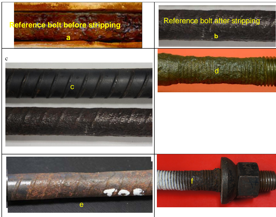
Figure 5 – Photos of parts of various corroded bolt sections compared with un- corroded section. Section (e) shows the evidence of crevice corrosion due to aeration at bolt end
