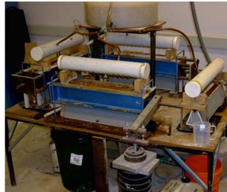
Figure 2 – Corrosion testing rig
