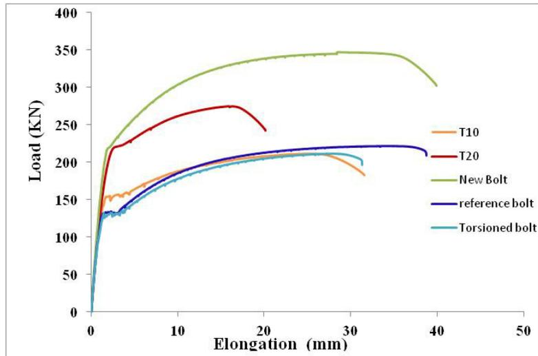
Figure 6 – Load displacement profiles of various bolts
