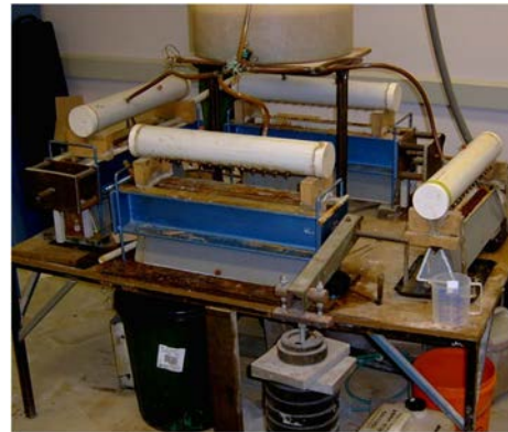
Figure 2 – Corrosion testing rig
