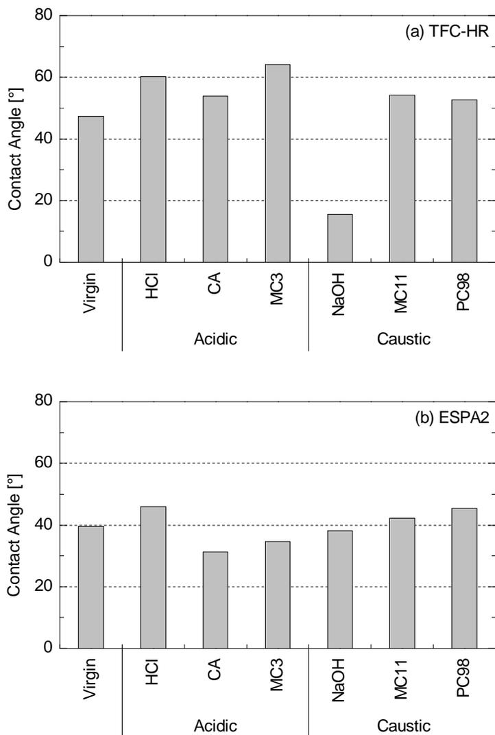
**Figure S4:** Hydrophobicity of the (a) TFC-HR and (b) ESPA2 membranes before and after being exposed to permeability of TFC-HR membrane before and after being exposed to cleaning solutions for 25 hours at 30 °C.
