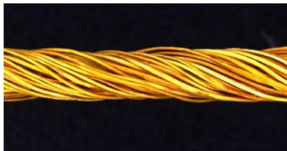
b) Twisted coir fibre drains
