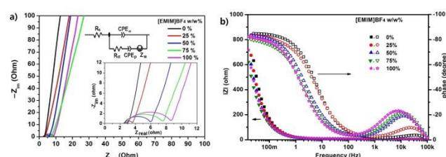
Fig. 6 (a) Nyquist plots for PVA/H<sub>3</sub>PO<sub>4</sub> and PVA/H<sub>3</sub>PO<sub>4</sub>/[EMIM]BF<sub>4</sub> supercapacitors (inset shows the magnified portion of high frequency part of Nyquist plot and the equivalent circuit of fit) and (b) the Bode plot for the PVA/H<sub>3</sub>PO<sub>4</sub> and PVA/H<sub>3</sub>PO<sub>4</sub>/[EMIM]BF<sub>4</sub> supercapacitors.
