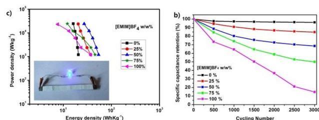
**Fig. 5** (a) Ragone plot of supercapacitor based on polymer gel electrolytes; the inset picture showing that three SCs in series can lighten up a blue LED (2.2 V, ~10-20 mA) powered by 30 s charged SCs and (b) Cycling stability of the supercapacitor for 3000 cycles charging/discharging.
