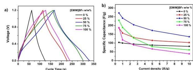
**Fig. 4** (a) Galvanostatic charge/discharge curve of PVA/H<sub>3</sub>PO<sub>4</sub> and PVA/H<sub>3</sub>PO<sub>4</sub>/[EMIM]BF<sub>4</sub> (25, 50, 75 and 100 wt. %) polymer gel electrolyte supercapacitors and (b) Variation of specific capacitance of SCs with respect to various discharge current densities.
