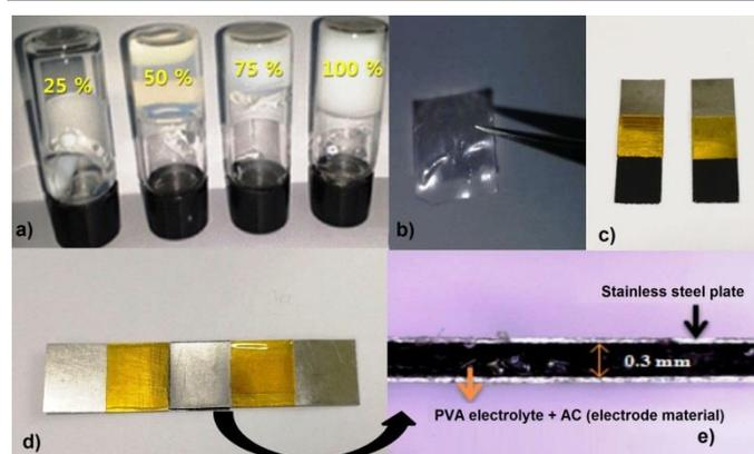
Fig. 1 (a) Photograph of PVA/H<sub>3</sub>PO<sub>4</sub>/[EMIM]BF<sub>4</sub> electrolytes, (b) PVA/H<sub>3</sub>PO<sub>4</sub>/[EMIM]BF<sub>4</sub> electrolyte film; (c) activated carbon electrodes; (d) fabricated full cell SC and (e) optical microscopic image of cross- section view.
