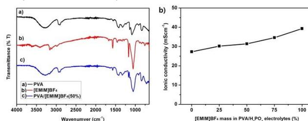
Fig. 2 (a) ATR-FTIR spectra of bare PVA, [EMIM]BF<sub>4</sub> and PVA/[EMIM]BF<sub>4</sub> (50%) polymer, (b) Ionic conductivity of PVA/H<sub>3</sub>PO<sub>4</sub>/IL polymer electrolyte at various wt.% of [EMIM]BF<sub>4</sub>.
