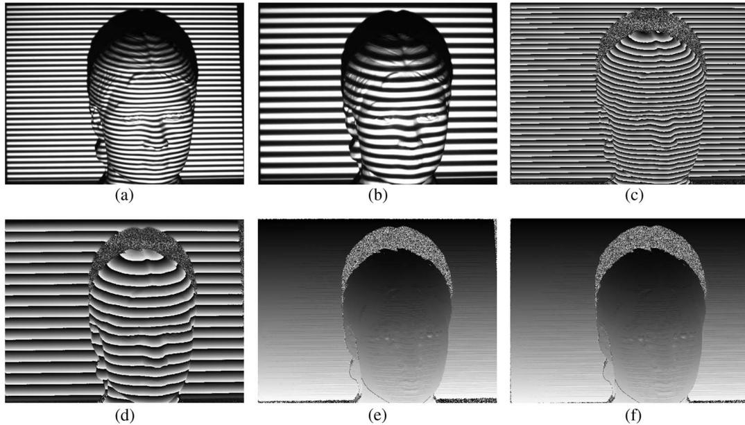
Fig. 1. Experiment results when  $\lambda_1 = 23$ ,  $\lambda_2 = 47$ . (a) and (b) are the deformed fringe patterns, (c) and (d) are the wrapped phase maps, (e) and (f) are the recovered absolute phase maps of (c) and (d).
