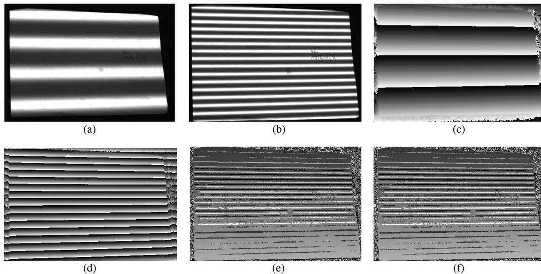
Fig. 2. Experiment results when  $\lambda_1 = 100$ ,  $\lambda_2 = 23$ . (a) and (b) are the deformed fringe patterns, (c) and (d) are the wrapped phase maps, (e) and (f) are the recovered absolute phase maps of (c) and (d).
