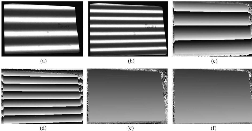
Fig. 3. Experiment results when  $\lambda_1 = 100$ ,  $\lambda_2 = 52$ . (a) and (b) are the deformed fringe patterns, (c) and (d) are the wrapped phase maps, (e) and (f) are the recovered absolute phase maps of (c) and (d).
