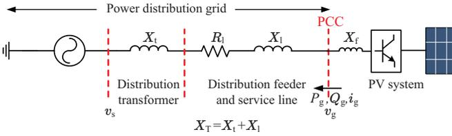
Fig. 1. Simplified model of the distribution grid.
