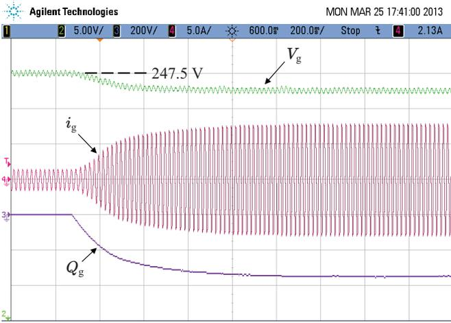
Fig. 9. Performance of the PCC voltage controller designed with a scaled integrator: Ch2: PCC rms voltage ( $V_g$ ) [5 V/div], Ch3: reactive power injected to the grid ( $Q_g$ ) [1 kVAR/div], Ch4: current injected to the grid ( $i_g$ ) [5 A/div].
