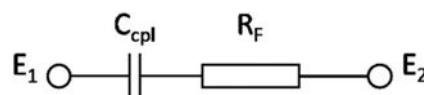
Fig. 1 Equivalent circuit diagram of a C^4D cell without stray and leakage capacitance. E_1 and E_2 are the excitation and pick up electrode, respectively. C_{cpl} symbolises the total coupling capacitance due to the fused silica wall and air surrounding the fibre. R_F is the resistance of the fibre.
