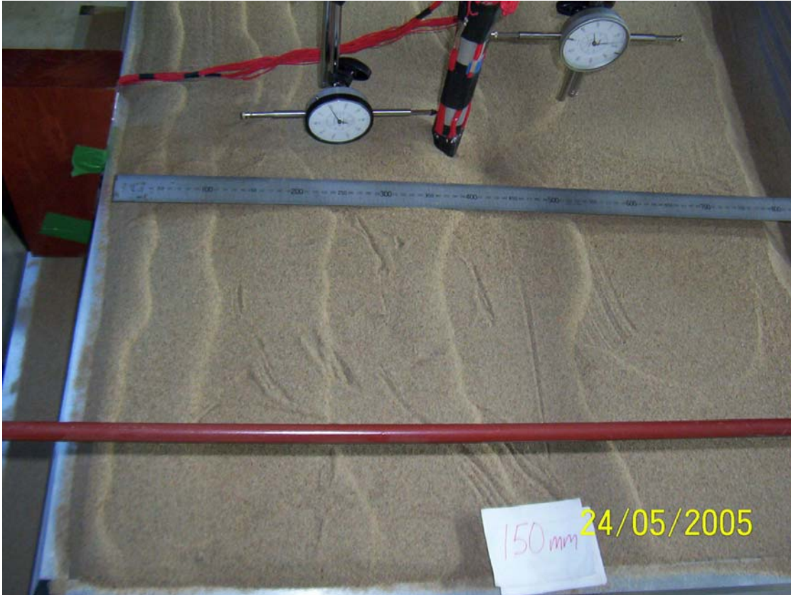
(h) Overview of sand heaves at w_f = 150 mm
