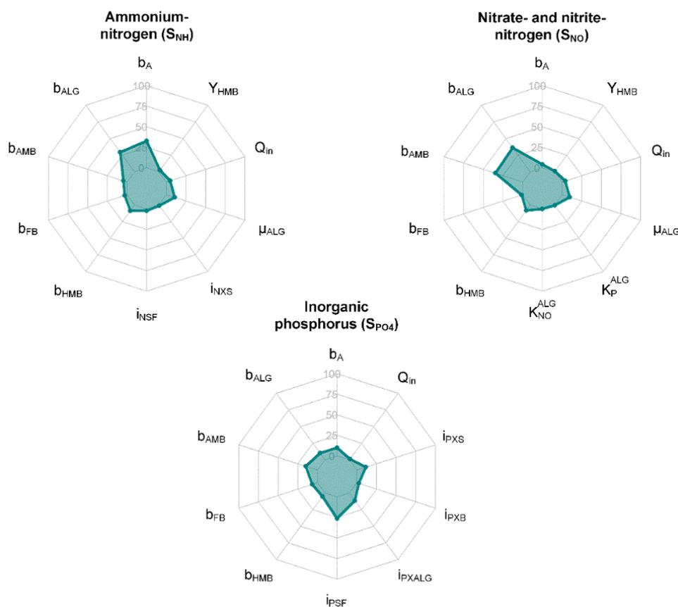
**Figure 4.** Ten most significant parameters influencing the variability of ammonium-nitrogen, nitrate- and nitrite-nitrogen, and phosphate in the waste stabilization pond (WSP) systems. The results in the radar graphs are the proportion of sensitivity function ( $s_{ij}$ ) for the state variable against the changes of each model parameter over the total sum of sensitivity measures. The description of the influential parameters in the graph can be found in the Supplementary Material F.
