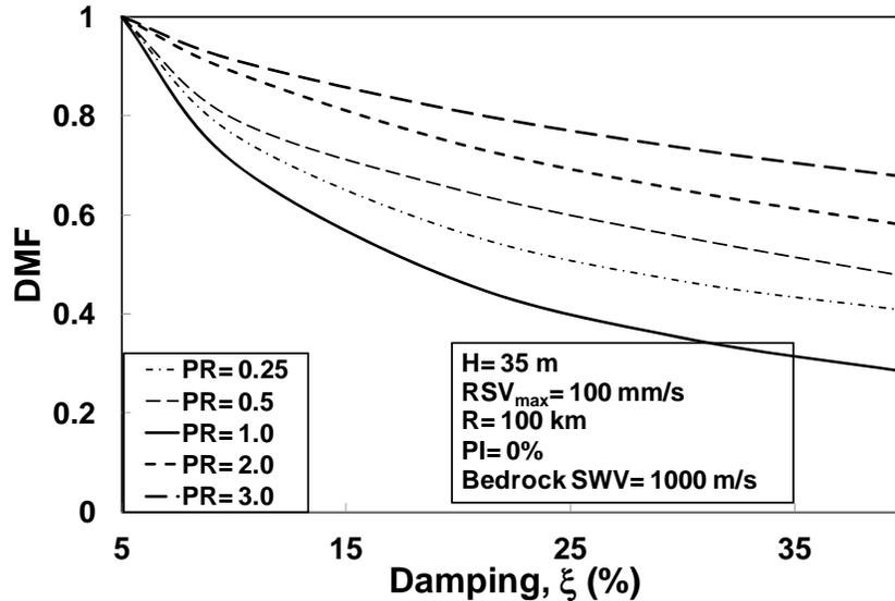
Figure 4: Influence of damping ratio ( $\zeta$ ) on DMF
