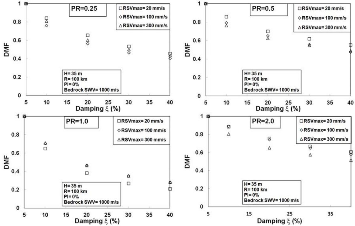
Figure 5: Influence of earthquake shaking level on DMF
