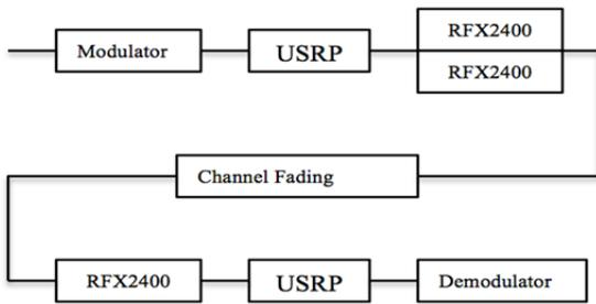
Fig. 1. The flowchart of the MIMO-STS systems SDR
