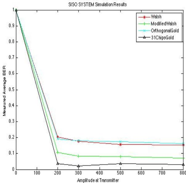
Fig. 2. Comparison of performance of modified walsh codes, orthogonal gold codes, 31 gold codes versus Walsh Hadamard codes in the presence of 1 MAI interferer at amplitude from 200 level to 500 level for randomly chosen chips delay from 1 to 9 on SISO systems
