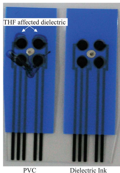
Fig. 8 Image of screen-printed electrodes after application of a thin film to the working electrode. The electrode array on the left has been coated with a PVC supported thin film while the right electrode array has been coated with a dielectric ink-supported thin film. The top two electrodes have had the film applied and allowed to evaporate; the bottom two electrodes have been gently scratched after the film was applied.
