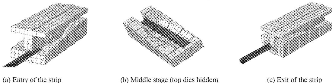
**FIGURE 4.** Millipede Forming process of U-channel
