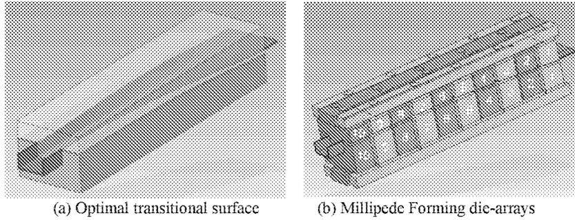
FIGURE 1. Concept of Millipede Forming method.
