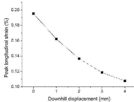
**FIGURE 3.** Effect of Downhill Displacement on Longitudinal Strain Reduction
