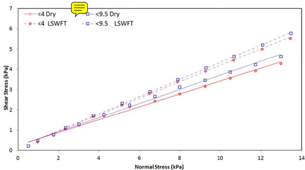
**Figure 8** – Wall Yield Loci for various particle size distributions of dry coal on SS304-2B tested on JST and LSWFT
