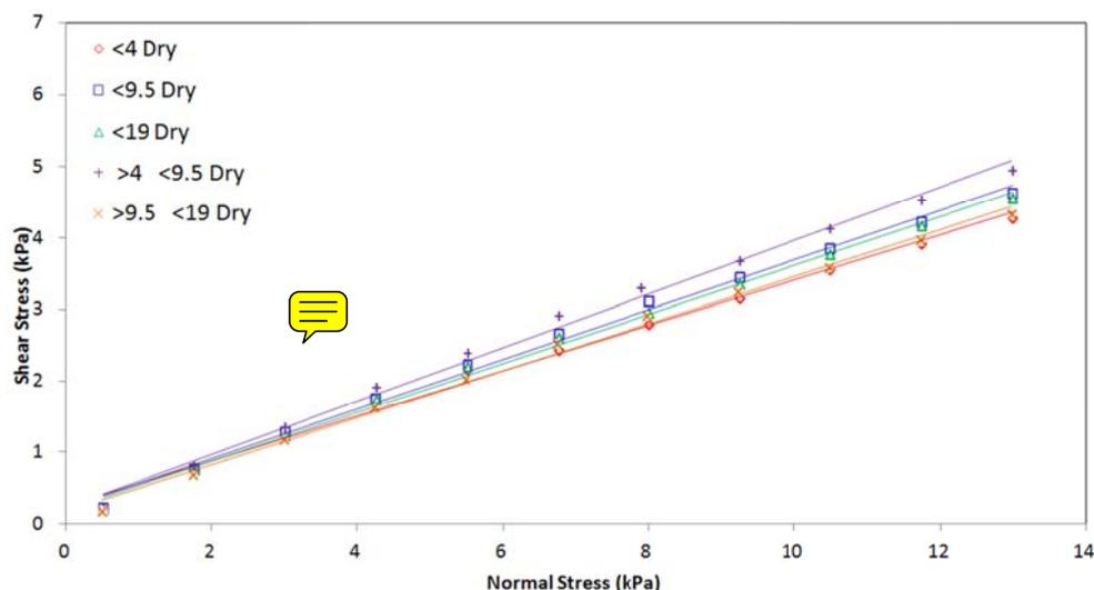
**Figure 4** – Wall Yield Loci for various particle size distributions of dry coal on SS304-2B
