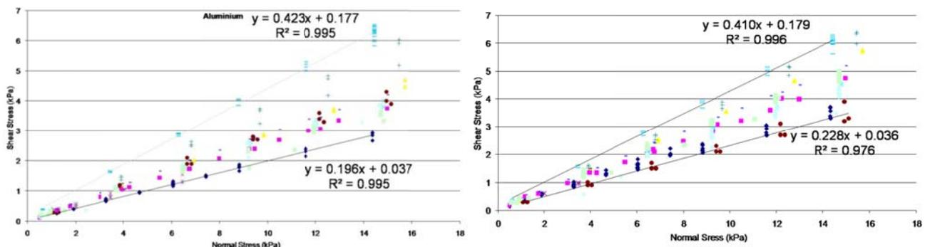
**Figure 2** – Wall Friction Angle vs Normal Stress for Acrylic Powder on Aluminium (Left) and Stainless Steel (Right) (McGee [9])
