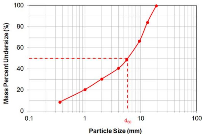
**Figure 3** – Particle size distribution of product coal sample
