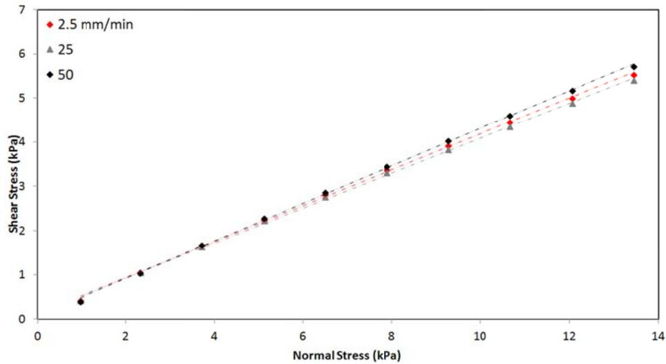
**Figure 10** – Wall Yield Loci of dry coal on SS304-2B tested on LSWFT at various shear rates
