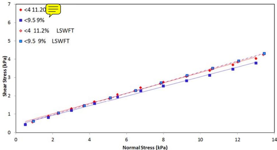
**Figure 9** – Wall Yield Loci for various particle size distributions of moist coal on SS304-2B tested on JST and LSWFT
