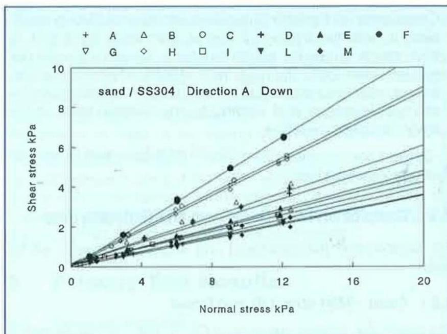
**Figure 1** – Wall Friction Measurements with Sand on SS304-2B (Haaker [5])
