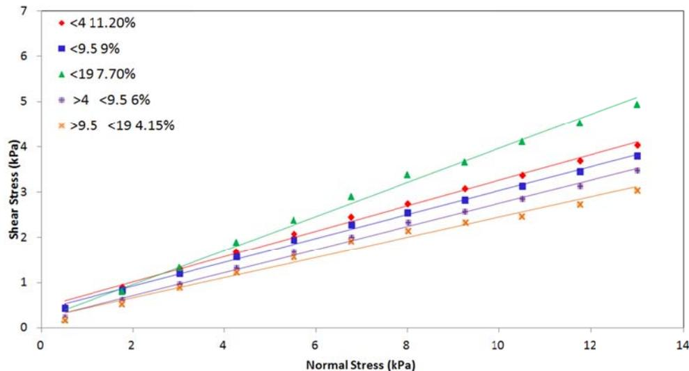
**Figure 5** – Wall Yield Loci for various particle size distributions of moist coal on SS304-2B
