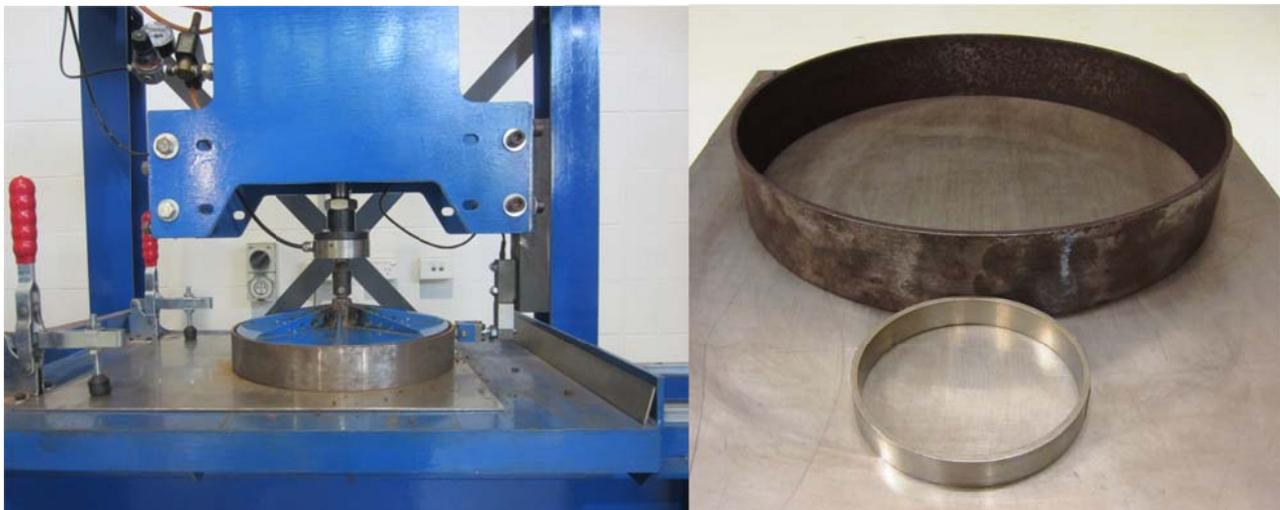
**Figure 7** – Setup of LSWFT (Left) and comparison of shear cell on JST and LSWFT (Right)
