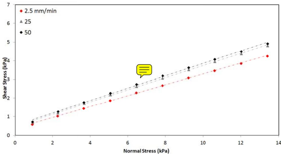
**Figure 11** – Wall Yield Loci of coal at 11.2% moisture content on SS304-2B tested on LSWFT at various shear rates
