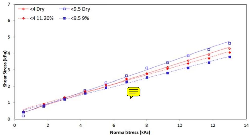
**Figure 6** – Wall Yield Loci for various particle size distributions of dry and moist coal on SS304-2B
