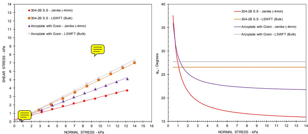
**Figure 12** – Wall Yield Loci (left) and wall friction angle,  $\phi_w$ , (right) of -4mm (4.1% moisture content) and bulk (3.6% moisture content) iron ore fines on SS304-2B and Arcoplate tested on JST and LSWFT
