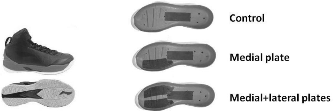
**Figure 1** — Test shoe conditions
