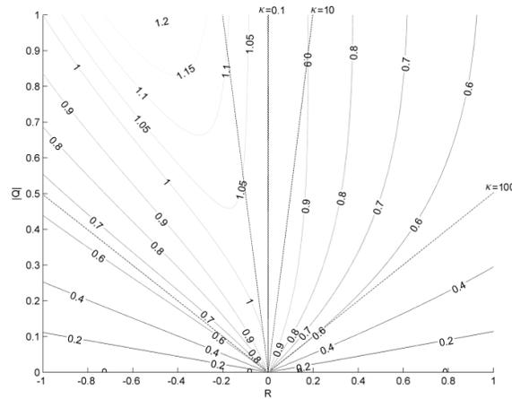
**Fig. 2.** Maximum fixed OWC power capture ratio for compressible and incompressible flow; the dashed lines represents the frequency response for the case  $\kappa=0.1$ ,  $\kappa=10$  and  $\kappa=100$  as indicated;  $\zeta=0.01$
