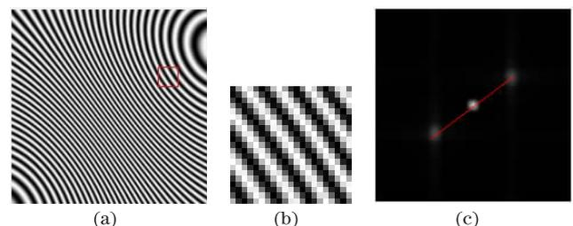
Fig. 1. Pictures of noise-free fringe patterns and the spectrum diagram of its local region. (a) Noise-free fringe patterns, (b) local region of the fringe patterns, and (c) Fourier spectrum of (b).
