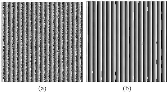
Fig. 6. Phase map of ESPI and its filtered image: (a) initial image, (b) filtered image by using the SOOPDE with the adaptive selective parameters.
