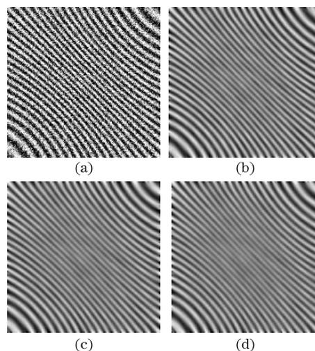
Fig. 3. Computer-simulated fringe pattern and its filtered image: (a) initial image, (b) filtered image by using the SOOPDE with  $\Delta t = 0.4$  and  $n = 38$ , (c) filtered image by using the SOOPDE with  $\Delta t = 0.4$  and  $n = 48$ , (d) filtered image by using the SOOPDE with  $\Delta t = 0.4$  and  $n = 58$ .
