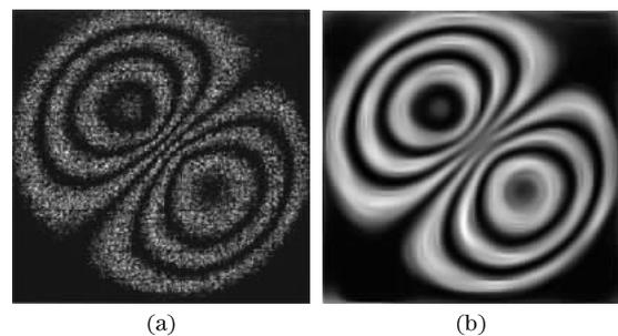
Fig. 5. Experimentally obtained ESPI fringe pattern and its filtered image: (a) initial image, (b) filtered image using the SOOPDE with the adaptive selective parameters  $\Delta t = 0.2$  and  $n = 137$ .
