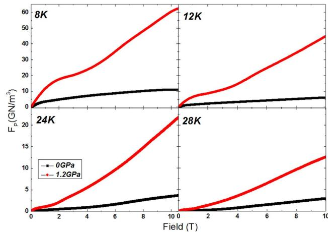
**Figure 3.**  $F_p$  versus field at 8, 12, 24, and 28 K at different pressures. At high fields and pressures, the  $F_p$  is found to be nearly 5 times higher at 8, 12, 24, and 28 K as compared to the corresponding value at  $P=0$  GPa, which agrees nicely with the  $J_c$  enhancement results.
