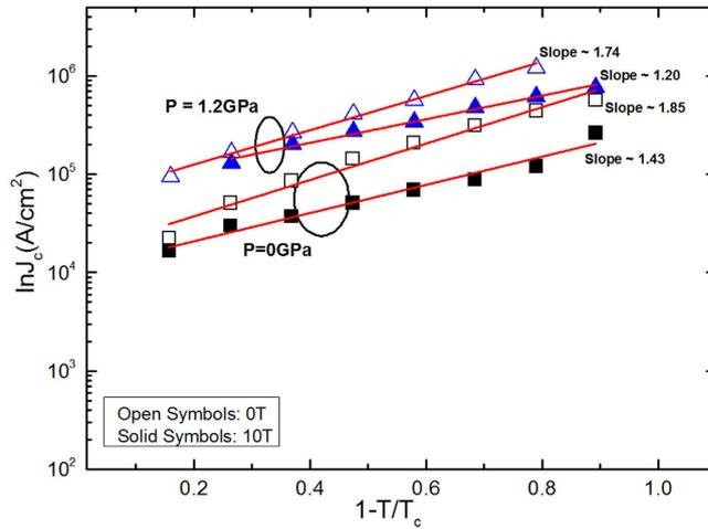
**Figure 6.**  $\ln J_c$  versus reduced temperature at different fields and pressures. The low  $\beta$  values at high pressure show the weak field dependences of  $J_c$  in contrast to its values at low pressure.
