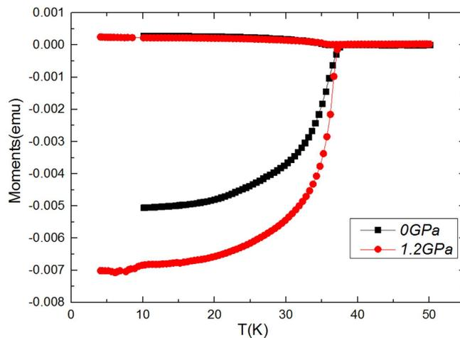
**Figure 1.** Magnetic moments vs. temperature at  $P = 0$  GPa and  $P = 1.2$  GPa.  $T_c$  remains almost unchanged at different pressures.  $T_c \approx 37.95$  K was found at  $P = 0$  GPa and  $P = 1$  GPa.
