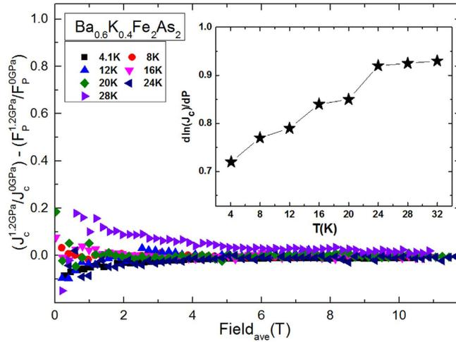
**Figure 5.**  $J_c - F_p$  ratios at  $P = 1.2 \text{ GPa}$  and  $P = 0 \text{ GPa}$ . The relative change of  $\ln J_c$  with pressure as a function of  $T$  is given in the inset. Analysis of the  $J_c - F_p$  ratios, acquired at different temperatures, leads to values of nearly zero. This result indicates that  $J_c$  enhancement is only related to pinning force enhancement.
