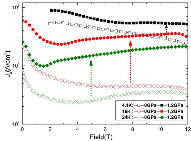
**Figure 2.**  $J_c$  as a function of field at  $P=0$  and 1.2 GPa at 4.1, 16, and 24 K.  $J_c$  is improved in both low and high fields and nearly five-fold  $J_c$  enhancement can be seen at 16 K and 24 K in both low and high fields at  $P=1.2$  GPa.
