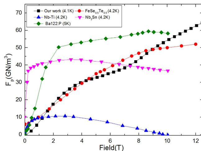
**Figure 4.** Comparison of  $F_p$  for different superconductors. Pressure can significantly improve  $F_p$  values to greater than  $60 \text{ GN/m}^3$  at  $H > 10 \text{ T}$ , which are even superior to those of  $\text{Nb}_3\text{Sn}$  and  $\text{NbTi}$ .
