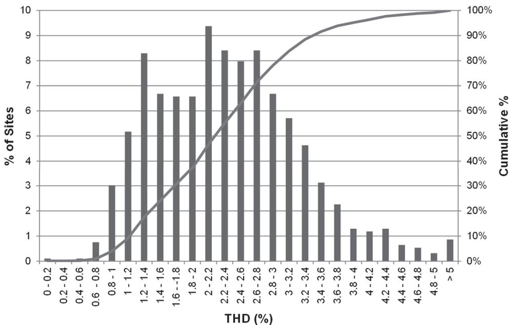
**Figure 7:** Histogram of MV voltage THD indices.
