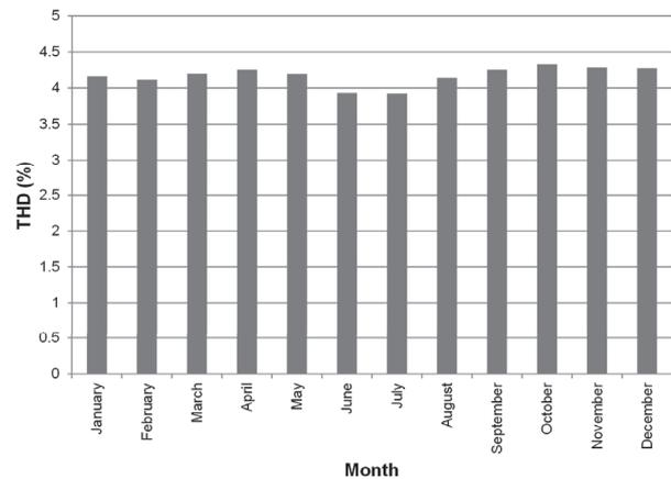
**Figure 4:** Monthly values of LV voltage THD for the 95<sup>th</sup> percentile site.
