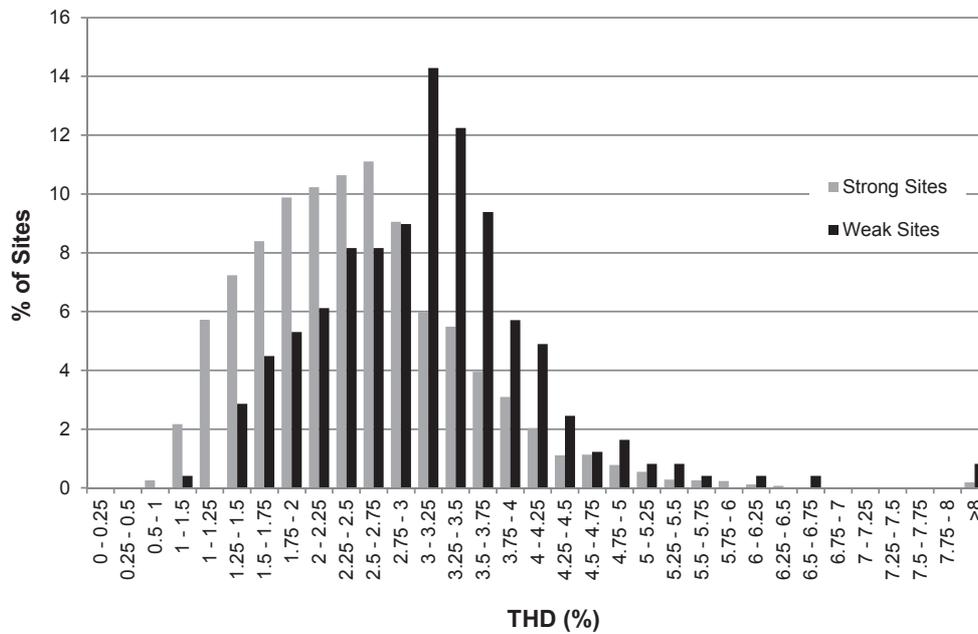
**Figure 2:** Comparison of voltage THD levels at strong and weak LV sites.
