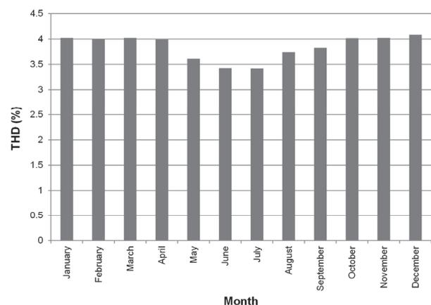
**Figure 9:** Monthly values of MV voltage THD for the 95<sup>th</sup> percentile site.
