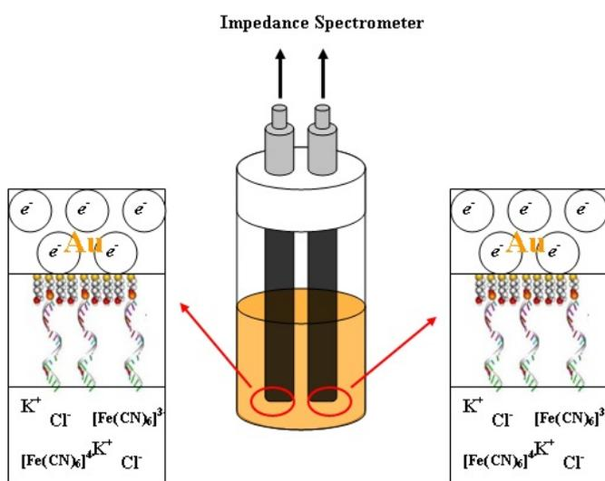
Figure 1: Two identically ssDNA/MCE modified gold electrodes used for analyte DNA detection in an electrochemical cell containing a solution of 5 mM ferrous/ferric cyanide and 300 mM KCl.
