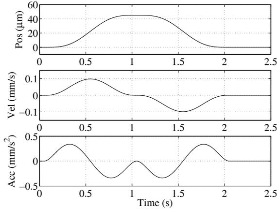
Fig. 4. 'Jerk-free' desired motion trajectory
