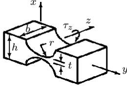
Fig. 2. Notch-type flexure hinge
