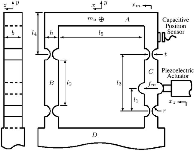
Fig. 1. Piezo-driven flexure-based four-bar micro/nano manipulator
