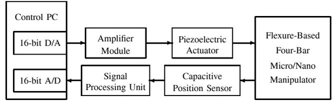
Fig. 3. Block diagram of the experimental architecture
