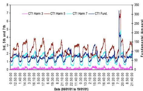
**Figure 4: Phase 'a' Fundamental, 3<sup>rd</sup>, 5<sup>th</sup> and 7<sup>th</sup> Harmonic current waveforms in site 2 (residential)**
