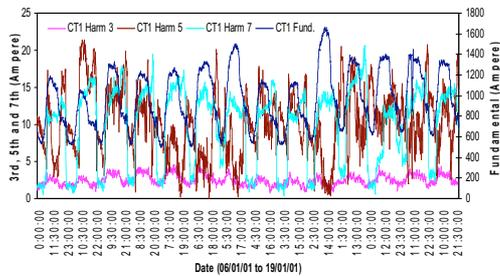
**Figure 3: Phase 'a' Fundamental, 3<sup>rd</sup>, 5<sup>th</sup> and 7<sup>th</sup> Harmonic current waveforms in site 1 (zone substation)**
