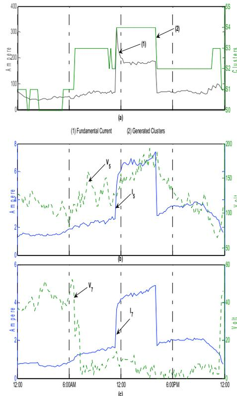
**Fig.10: Overload on residential feeder due to transferring load from faulty feeder (a) Clusters superimposed on the fundamental current waveform, (b) 5<sup>th</sup> harmonic current and voltage data, (c) 7<sup>th</sup> harmonic current and voltage data**
