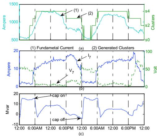
**Figure 6: Clusters at substation site in two working days (a) Clusters superimposed on the fundamental current waveform.. (b) 7<sup>th</sup> harmonic current and voltage data. (c) MVar load at the 33kv busbar.**
