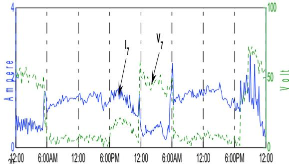
**Figure 7: 7<sup>th</sup> harmonic current and voltage at Commercial site in two working days**
