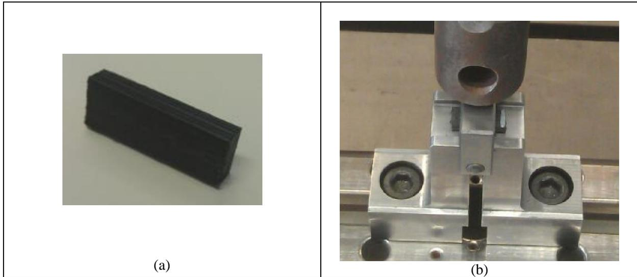
Figure 3. (a) Test coupons; (b) Experimental set-up for the ILSS test using Instron 50KN.
