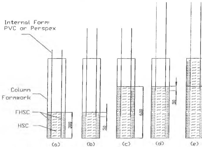
Figure 2 Column casting procedure
