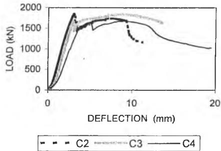
Figure 7 Columns C2, C3 and C4 – Varying fibre location (Constant fibre content of 0.1%)
