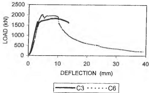
Figure 5 C3 and C6 - Varying fibre content (Fibres located in cover plus extending into the core)
