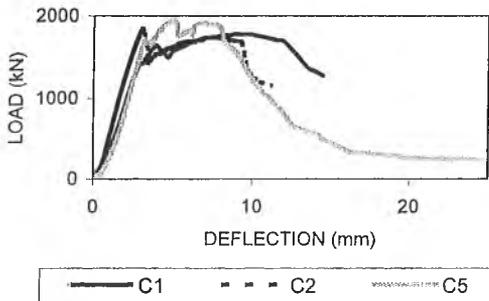
Figure 4 C1, C2 and C5 - Varying fibre content (Fibres located entire cross-section)
