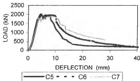
Figure 8 Columns C5, C6 and C7 – Varying fibre location (Constant fibre content of 0.3%)
