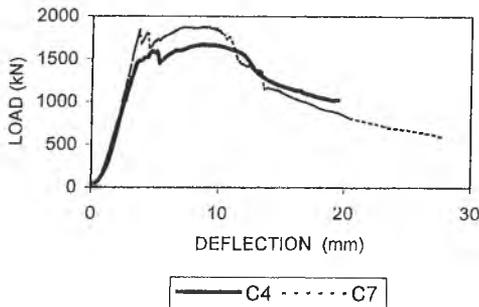
Figure 6 C4 and C7 - Varying fibre content (Fibres located in cover only)
