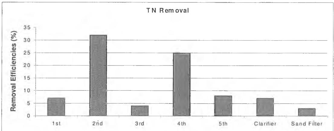
Figure 5: TN removal efficiencies in each chamber
