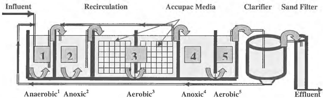
**Figure 1: Schematic of the 5 stage biological reactor with Final Clarifier and sand filter polishing**
