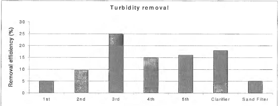
Figure 4: Turbidity removal efficiencies in each chamber
