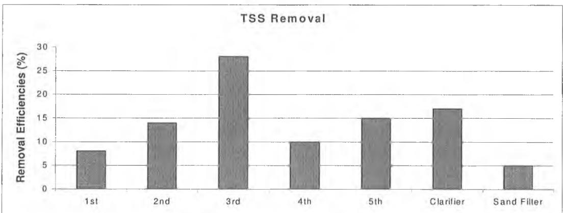
Figure 3: TSS removal efficiencies in each chamber
