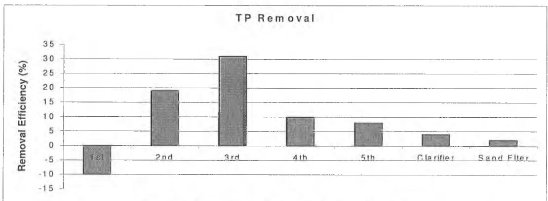
Figure 6: TP removal efficiencies in each chamber
