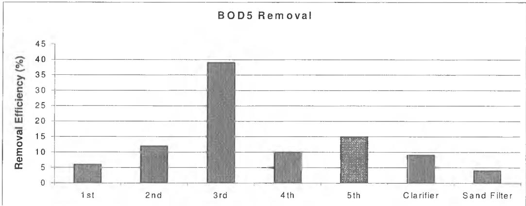
Figure 2: BOD<sub>5</sub> Removal efficiencies in each chamber
