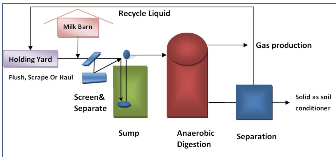
**Figure 3: Integration of Anaerobic Digestion in Dairy Waste Management Practice**
