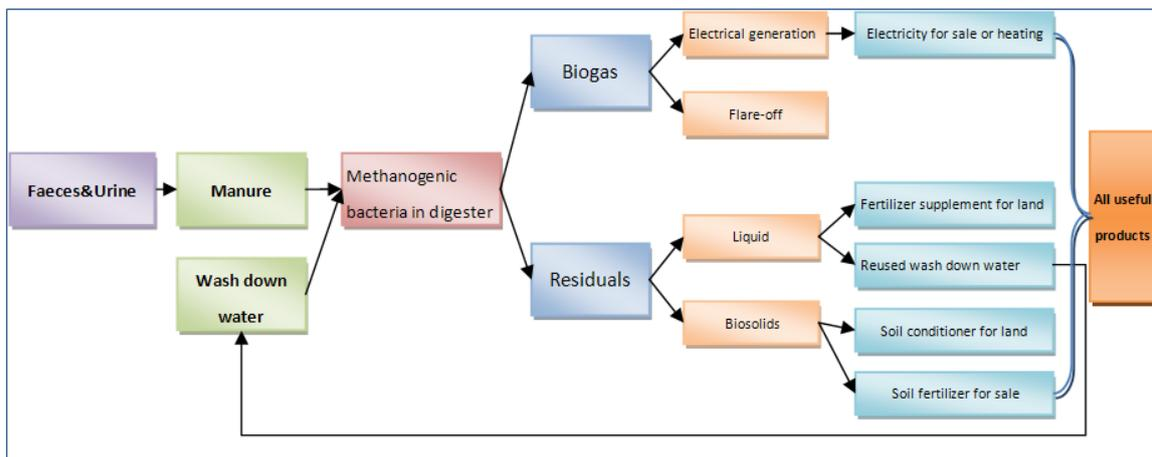
**Figure 1: Anaerobic digestion process of dairy manure**
