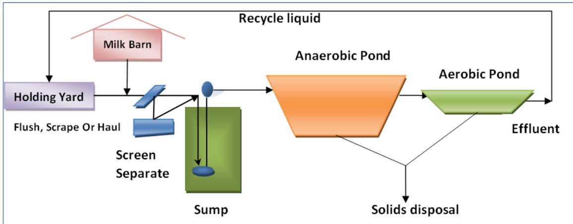
**Figure 2: Dual-pond system with effluent recycled for flood washing**
