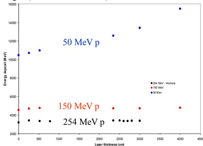
Fig. 4 Energy deposit in the sensors as a function of the lid thickness, resulting from simulated irradiation with protons at various energies (254, 150 and 50 MeV).
