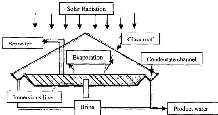
Figure 1: Design of a simple solar still (Duffie & Beckman, 1991)
