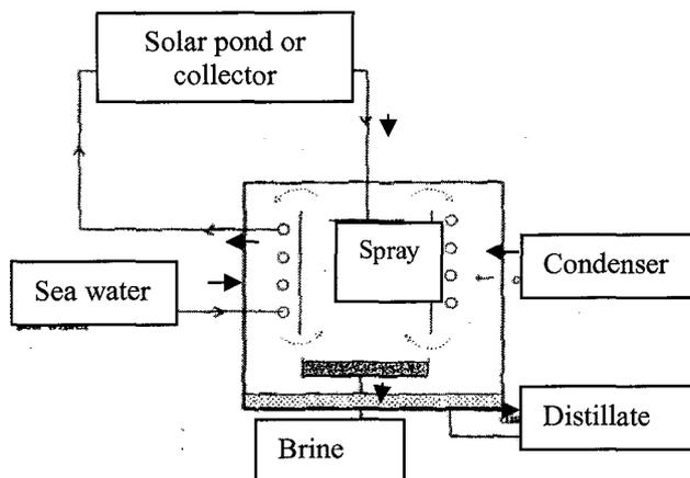
Figure 3: Spray-type evaporator (Joyce et al, 1994)
