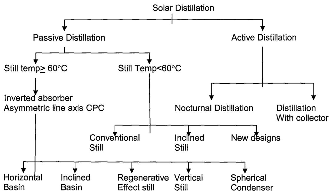
Figure 2: Taxonomy of solar distillation development (Tiwari et al, 1994)
