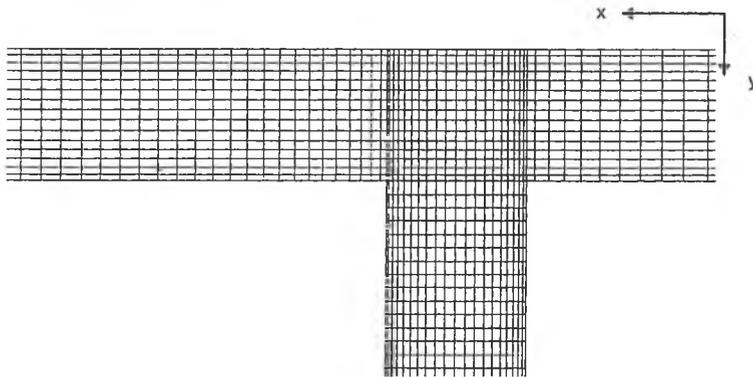
Figure 5. Computational Mesh – Detail near junction
