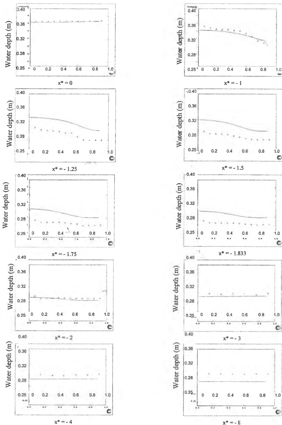
Figure 12. Water Depth Comparisons at Various Locations ( $\square$  Experiment; — Simulation);  $x^* = x/w$ , where  $w$  = width of the channel and  $x$  = distance along the main channel in the experimental channel.
