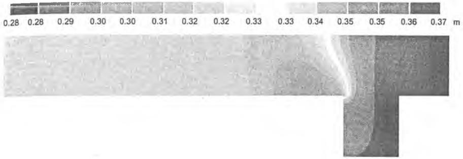
Figure 10. Computed Water Depth contours near Junction using PHOENICS
