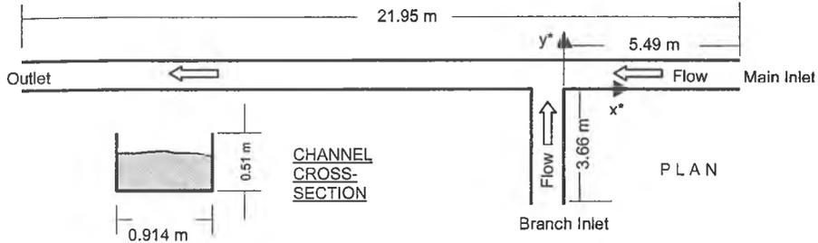
Figure 2. Schematic of Experimental Arrangement (Weber et al, 2001)
