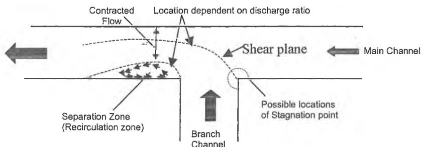
Figure 1. Flow Characteristics in Open Channel Junction (Weber, et al, 2001)
