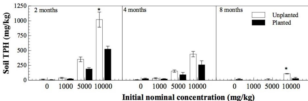
**Figure 2:** Soil TPH concentration (mg/kg) in planted (*P. foliosa*) and unplanted soil at time intervals 2, 4 and 8 months for the range of initial nominal SAB fuel concentrations. Data are mean  $\pm$  SEM, n = 5. \* indicates significant difference between planted and unplanted treatments at p = 0.05 across concentrations, within each sample interval.
